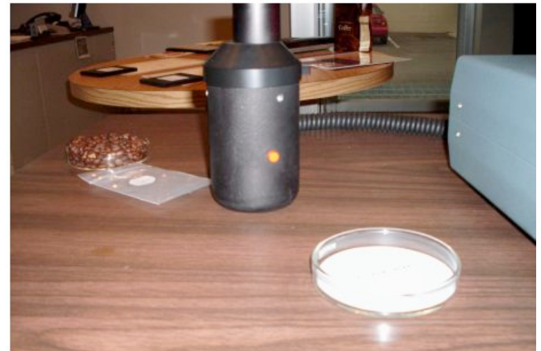
Place sample dish on Search Unit Press orange button to display SCAA Classification Number
